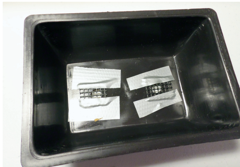
Figures 6 & 7: Below, A plastic bonsai pot is used for the experiments. Drainage holes are covered with mesh as usual from the inside, held here with duct tape instead of wire. The holes are sealed on the bottom with a temporary strip of duct tape, which is removed to allow the pot to drain. Photo credits: Brian Heltsley.
